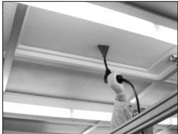
Figure 15: Probe Testing a Clean Room Ceiling
